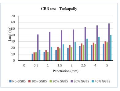
Fig.8: CBR values with GGBS for Turkapally soil sample
