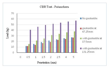
**Fig.7:** CBR values with geotextile for Patancheru soil sample From both the graphs it is seen that, the CBR value is maximum when the geotextile is placed at 131.25mm height **CBR Test for GGBS**
