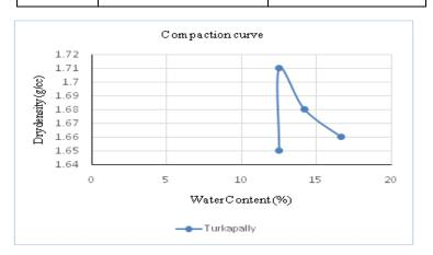
**Fig 4:** Compaction graph for Turkapally soil sample from the graph MDD is 1.71[g/cc] and OMC is 12.5[%]
