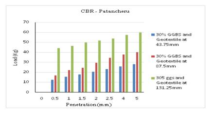
Fig 10: CBR values with a combination of GGBS and geotextile for Turkapally soil sample
