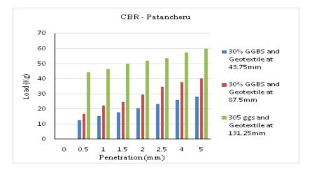
**Fig 11**: CBR values with a combination of GGBS and geotextile for Patancheru soil sample From both the graphs it is to observed that, the CBR values of the soil samples is maximum when it is mixed in combination with 30% GGBS and geotextile placed at 131.25mm height
