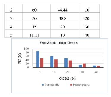
Fig .3: FSI values of different % of GGBS for two soil samples
